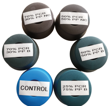
Figure 3: Cap samples produced using different compositions of virgin and AHP recycled plastic
